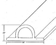
**Application:** On wood structures, nail with large-headed aluminum or stainless steel nails, 4 inches on center of top and bottom flanges. On metal structures, use stainless steel or aluminum sheet metal screws and washers.
