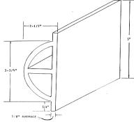
**Application:** On wood structures, nail with large-headed aluminum or stainless steel nails, 4 inches on center of top and bottom flanges. On metal structures, use stainless steel or aluminum sheet metal screws and washers.
